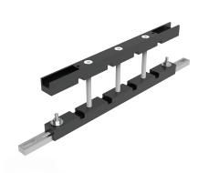
**Beschreibung:** Busbar support up to 1600A to be mounted horizontally or vertically. Mounts directly to the enclosure frame or with help of CLPF profiles. Available in single and double bar per phase for bar thickness 5 mm and only single bar per phase for bar thickness 10 mm, and width from 25 to 80 mm.
