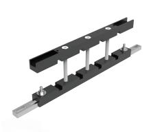
**Kuvaus:** Busbar support up to 1600A to be mounted horizontally or vertically. Mounts directly to the enclosure frame or with help of CLPF profiles. Available in single and double bar per phase for bar thickness 5 mm and only single bar per phase for bar thickness 10 mm, and width from 25 to 80 mm.
