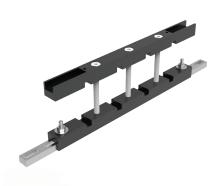
**Description:** Busbar support up to 1600A to be mounted horizontally or vertically. Mounts directly to the enclosure frame or with help of CLPF profiles. Available in single and double bar per phase for bar thickness 5 mm and only single bar per phase for bar thickness 10 mm, and width from 25 to 80 mm.
