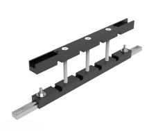
**Omschrijving:** Busbar support up to 1600A to be mounted horizontally or vertically. Mounts directly to the enclosure frame or with help of CLPF profiles. Available in single and double bar per phase for bar thickness 5 mm and only single bar per phase for bar thickness 10 mm, and width from 25 to 80 mm.
