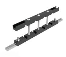
**Popis:** Busbar support up to 1600A to be mounted horizontally or vertically. Mounts directly to the enclosure frame or with help of CLPF profiles. Available in single and double bar per phase for bar thickness 5 mm and only single bar per phase for bar thickness 10 mm, and width from 25 to 80 mm.
