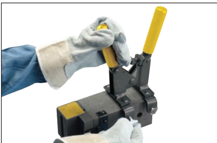
Fig. 7 – Tighten the clamp thumbscrews onto the mold.
