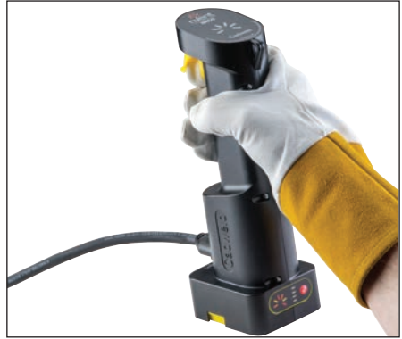
Fig. 13 – Using the control unit, lift the trigger cover and press the ignition button and hold. You will see the 6 lights on the top of the control unit light up as it is charging. After the 6th light is illuminated, the control unit will send a charge to the ignition strip, initiating the Cadweld Plus exothermic reaction.
