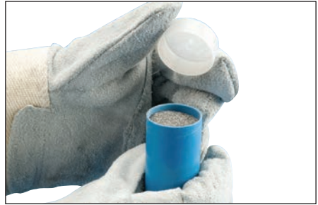
Fig. 19 – Remove the lid over the mold crucible.
