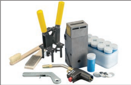
Fig. 2 – Gather the proper materials and equipment for the type of connection you are making. The typical Cadweld system requires a graphite mold, handle clamp, welding material, natural bristle brush for mold cleaning, wire brush for cleaning/preparing conductors, flint igniter, and propane torch.
