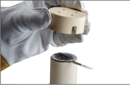
Fig. 10 – Place the ceramic lid onto the mold.
