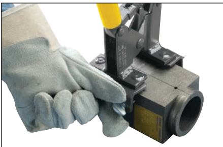
Fig. 7 – Tighten the clamp thumbscrews onto the mold.
