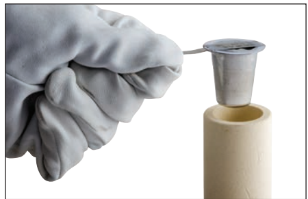
Fig. 9 – Place the welding material cup into the top of the mold. Make sure the ignition strip nests into the recess on the top edge.
