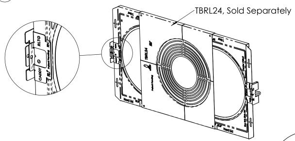
Tighten (1) Screw on Each RLTG (Both Ends)
