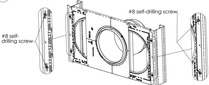
Adjust Center Plate and Tighten at Least (1) Screw on Center Plate to Prevent Any Movement of Center Plate
