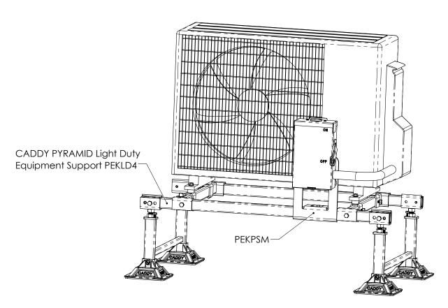
Can Prefab PEKPSM Complete (Power Switch Box, Wires, Conduit, etc.) Before Install on Site
