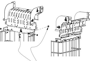
FOR ADDED SECUREMENT, ASSEMBLE (QTY-6) STANDARD 1/4"-20 CARRIAGE BOLT/HEX NUT(S) (NOT INCLUDED'
