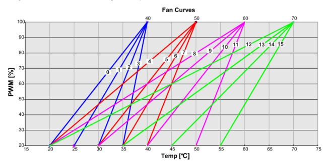
The temperature curve can be selected via the DIP switch SW100 or SMBus. The fan speed can also be set manually between 25 % and 100 % via SMBus.
