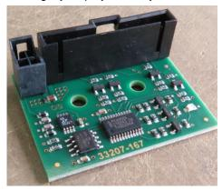
The current display Part No.: 23207-168 with 6 SMD LEDs
