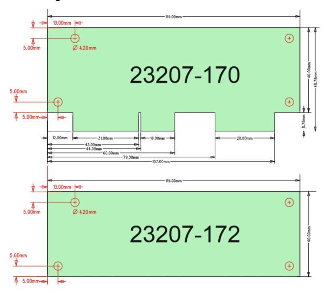
To mount the FCM3 inside a system, Schroff recommends to use locking supports, as example ETTINGER Part No.: 006.27.086
