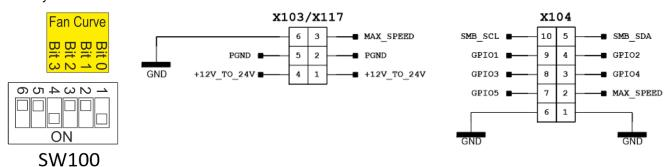
If the MAX\_SPEED pins on connector X103/117 or X104 are connected to GND, the fans rotate permanently at 100 %.
