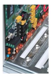
The Series NW126 is an economical PCB retention solution for cold wall applications. Constructed of rugged stainless steel, the independent spring design provides board retention for low shock and vibration applications.
