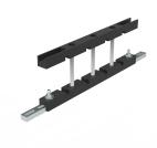
This busbar support, ECBS, is available for one or two bars up to  $80 \times 5$  mm or one bar up to  $80 \times 10$  mm. The support can be mounted both horizontally and vertically. It is available off the shelf and tested according to IEC 61439.
