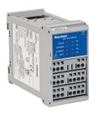
nVent RAYCHEM NGC-40 Series - IO Module provides up to four additional RTD inputs. These can be assigned to any NGC-40-HTC/HTC3 module. It also provides one alarm relay that can be connected to an external annunciator and one digital input that is programmable and may be assigned to any NGC-40-HTC/HTC3 module for various functions such as forcing the contactor or SSR on or off.
