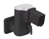
Syspend 180-Max Horizontal Wall Joint mounts the suspension system to a vertical surface, allowing the tube to extend horizontally. The arm can be rotated 300 degrees. Includes a safety stop and maintenance-free bearings.
