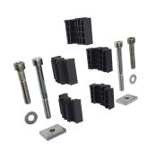
High short-circuit kit designed to upgrade the nVent ERIFLEX IFBS so it may withstand high short-circuit values up to 130kA peak. This kit includes two strut nuts, two M8 – CHC Head Screws (75mm), two M8 – CHC Head Screws (40mm), and five reinforced spacers.
