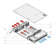
VME64x system for 2 horizontally mounted VME64x boards 6 U, 160 mm. Rear I/ O option. The power for the system is supplied by an open frame power supply. A hot swap fan tray with 4 fans guarantee an excelant cooling.
