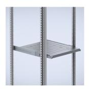
This shelf, that is mounted on 19" profiles, can be extracted to allow for the inspection and maintenance of installed components. It has ventilation openings to ensure for proper air circulation within the enclosure.
