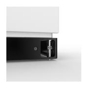
The adjuster has been designed for levelling on uneven floors at the installation site. Levelling range is up to a maximum of 15 mm and it is installed on the assembled enclosure through the PF/PFS plinth corner piece.
