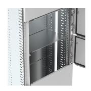
This steel zink plated separation plate, MSESM, is available off the shelf and pre-sized. The plate should be used when subsections need to be segregated. It is placed between a mounting plate and the doorway for partial doors. No screws are needed, which makes mounting easy. The fix section can then comply to up to form 4 segregation according to IEC 61439.
