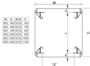
Varistar welded steel frame for static load requirements. For 19", ETSI or mounting plate integration. For mobile applications.
