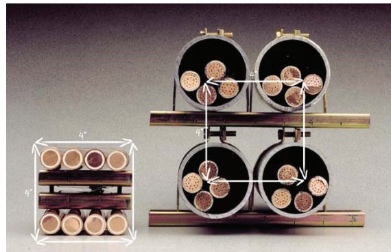
500 kcmil: At 75 C = 620 Amps MI vs. RHW/THHN 380 Amps
