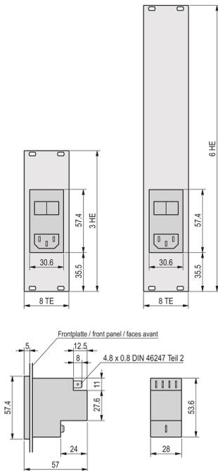
Front Panel for CompactPCI Systems with mounted Wide Range AC Input Module containing AC Plug, Fuse Holder and EMC Filter.
