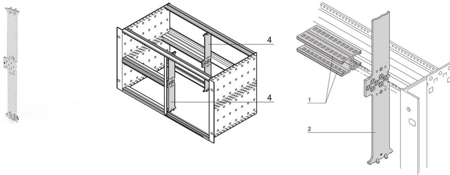
The support is bolted into the grid holes of the horizontal rails and allows a split of a 6 U subrack in 2 x 3 U parts.
