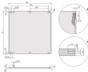
Flat front panel. Shieldable with stainless steel EMC gasket.
