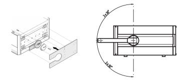
The assembly kit must be used if a tip-up handle should be mounted. Standard side covers should be replaced.
