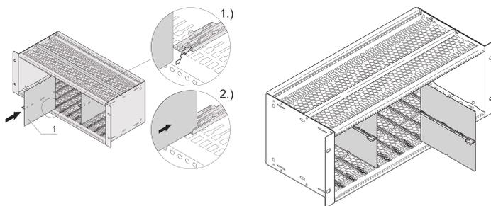
Splitting kit is inserted into the appropriate receptacle of the nVent SCHROFF MicroTCA guide rail and locks into the appropriate stud of the guide rail.
