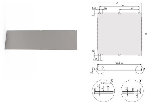
U-profile front panel for textile EMC gasket.
