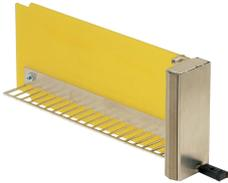
This AdvancedMC filler module consists of a stainless steel front panel without LEDs and has EMC gaskets on the left hand and bottom side. The filler module is fixed into the chassis card guide by a snap in plastic nose. The module can be used to cover an empty slot, to ensure EMC shielding and close the front to seal air leaks into the chassis. These filler modules can be used in AdvancedMC Carriers and in MicroTCA slots. It doesn't require a locking bar.
