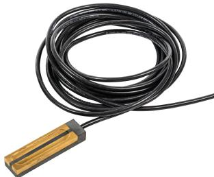
nVent RAYCHEM RAYSTAT-M2-R-SENSOR is a moisture detector designed for mounting in gutters and drain pipes. It is used with the RAYSTAT-M2 thermostat and RAYSTAT-M2-A-SENSOR for roof and gutter de-icing applications.
