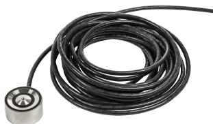
nVent RAYCHEM RAYSTAT-M2-G-SENSOR is a ground temperature and moisture sensor designed for embedding into the surface of the outdoor area. It is used with the RAYSTAT-M2 thermostat to ensure the heating system is only energized when the surface temperature is below the selected setting and snow or ice is present on the sensor.
