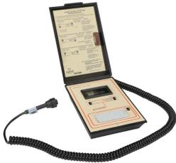
nVent RAYCHEM TraceTek TT-PTB-1000 is a battery powered portable device for testing individual lengths of sensing cable, up to 1000 m / 2000 ft. Useful for installation and maintenance of extensive systems.
