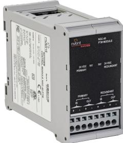
nVent RAYCHEM NGC-40 Series - Power Termination Module accepts a primary and redundant power supply input, also accepts CAN bus inputs and provides for termination of the CAN bus. Each NGC-40-PTM can provide power for a maximum of 10 NGC-40 modules.
