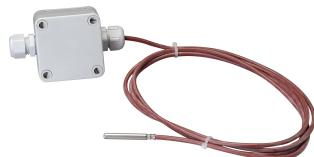
nVent RAYCHEM MONI-PT100-NH sensor is a two-wire platinum resistance temperature detector (RTD), supplied with glass fiber reinforced polycarbonate junction box, for non-hazardous areas.
