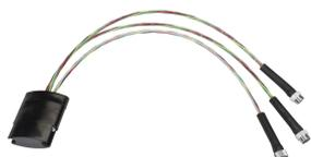
nVent RAYCHEM TraceTek TT-MBC-MC is a modular branch connection, with metal connectors, used to create T-branches in sensor circuits. Contains weighted resistors that simulate 4.5 m / 15 ft of sensing cable on the end and branch legs.
