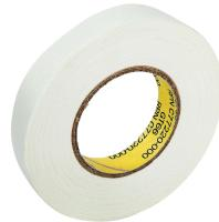
nVent RAYCHEM GT-66 is a glass installation tape to attach trace heating cables to pipes. For use on stainless steel, or when installation temperatures drop below 40 °F / 5 °C, use GS-54 fixing tape. AT-180 / ATE-180 aluminum tape is used to attach heating cables and thermostat sensors to pipes and tanks.
