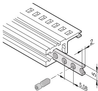
The threaded insert is a metal strip with thread M2.5 and allows the fixing of front panels.
