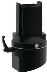
Use Angled Coupling Tilted Forward to mount enclosure at a 15-degree forward angle. Enclosure can be rotated 300 degrees and locked in position. Includes safety stop and maintenance-free bearing.
