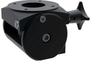
Suspend 281-Max Angle Adapter enables enclosure angle to be adjusted forward or backward up to 30 degrees. Must be used in conjunction with a coupling (not compatible with S2MFC48). Maximum load bearing capacity is 67 lb. (30.4 kg).
