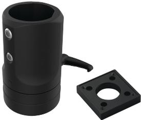
Syspend 281-Max 48-mm Round Tube Flange Coupling attaches the Vertical Motion Pedestal Tube or any 48-mm round tube to the enclosure. Enclosure can be rotated 300 degrees and locked in position. Includes safety stop and maintenance-free bearing.
