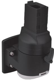
Suspend 180-Max Vertical Panel Coupling mounts a vertical tube to the back of an enclosure or screen using Video Electronics Standards Association (VESA) mounting. The coupling has mounting holes drilled for standard VESA 75 and 100 flange sizes. It enables the enclosure to rotate 300 degrees and can be locked into a given position. The vertical panel coupling has a safety stop and maintenance-free bearings.
