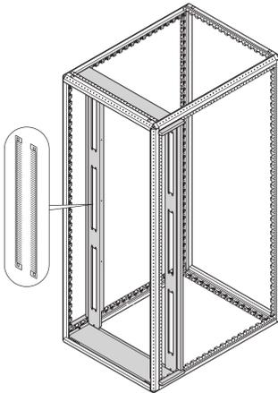
Brush strip to close 2 U by 19" cutouts for air management blanking panels. Square hole mounting with cage nuts.
