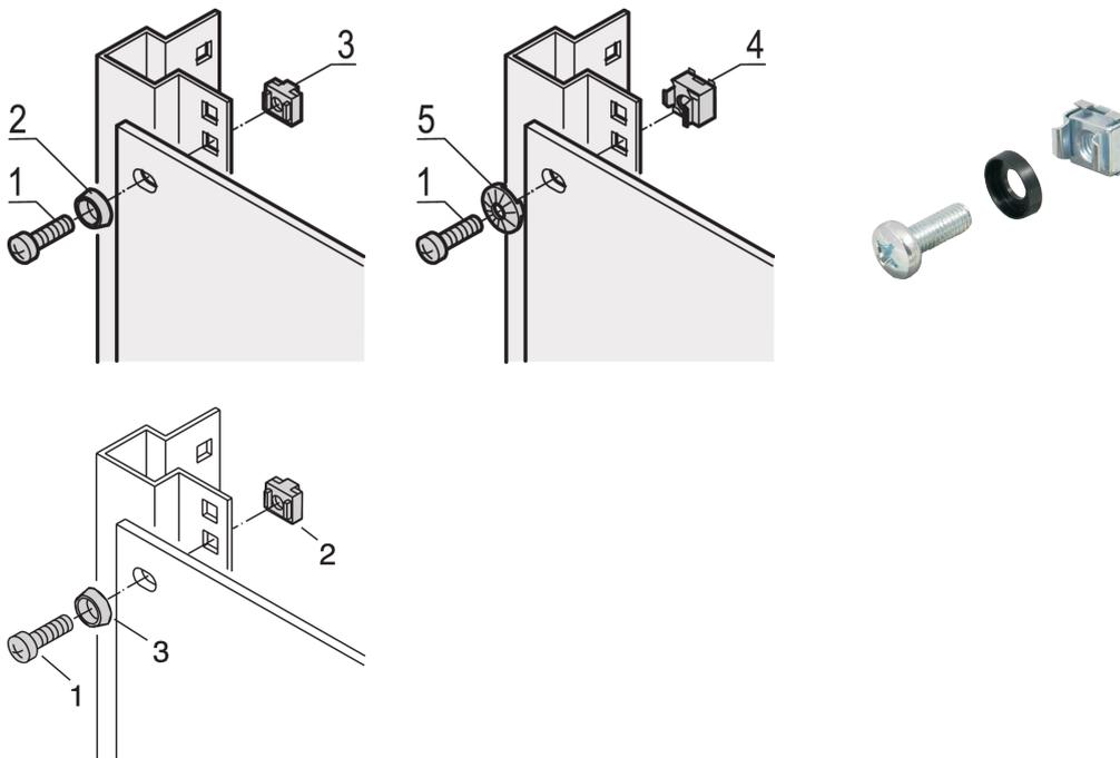
For standard grounding use a grounding nut and washer on at least one attachment point.
