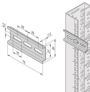
DIN rail for thermostat or hygrostat clamping.
