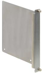
To cover unused AdvancedMC, MCH or PM slots in MTCA.1 and MTCA.4 systems or unused slots in a MTCA.0 system with locking bar. Modules consist of a front panel with latches and captive screws, EMC gasket and side panel. Modules can be fixed to the card cage with the captive screws.
