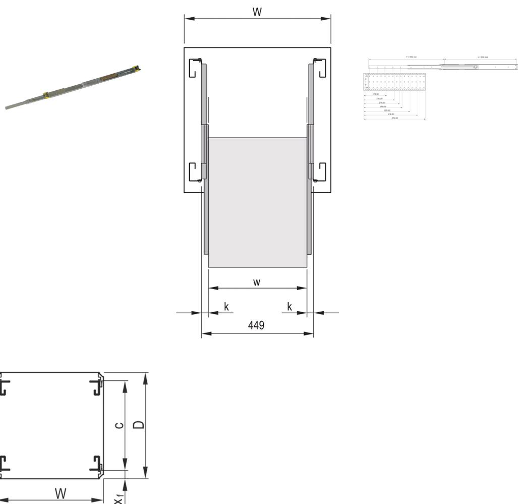
Narrow Telescopic Slide for Subracks with > 100 % extension.
