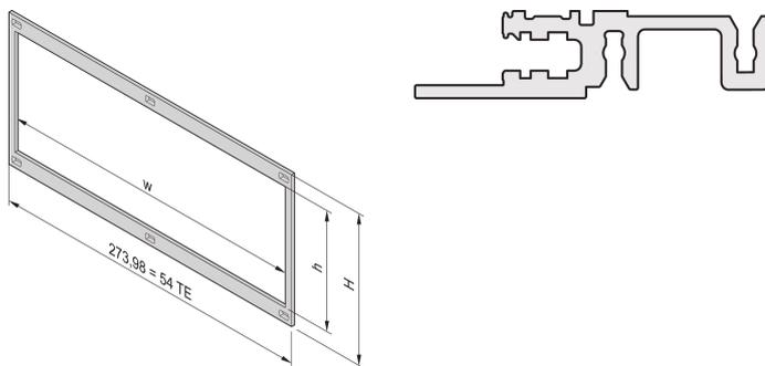
Front frame installation provides the contact between subracks and assemblies. It must be used if a customer has selected a horizontal board mounting Kit.
