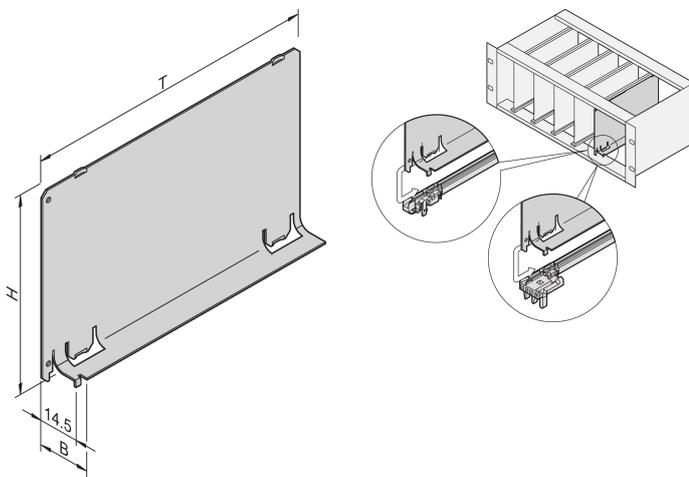
The air baffle without a partial front panel can be combined with a front panel that covers the complete width. It covers an empty slot to eliminate an air leak.
