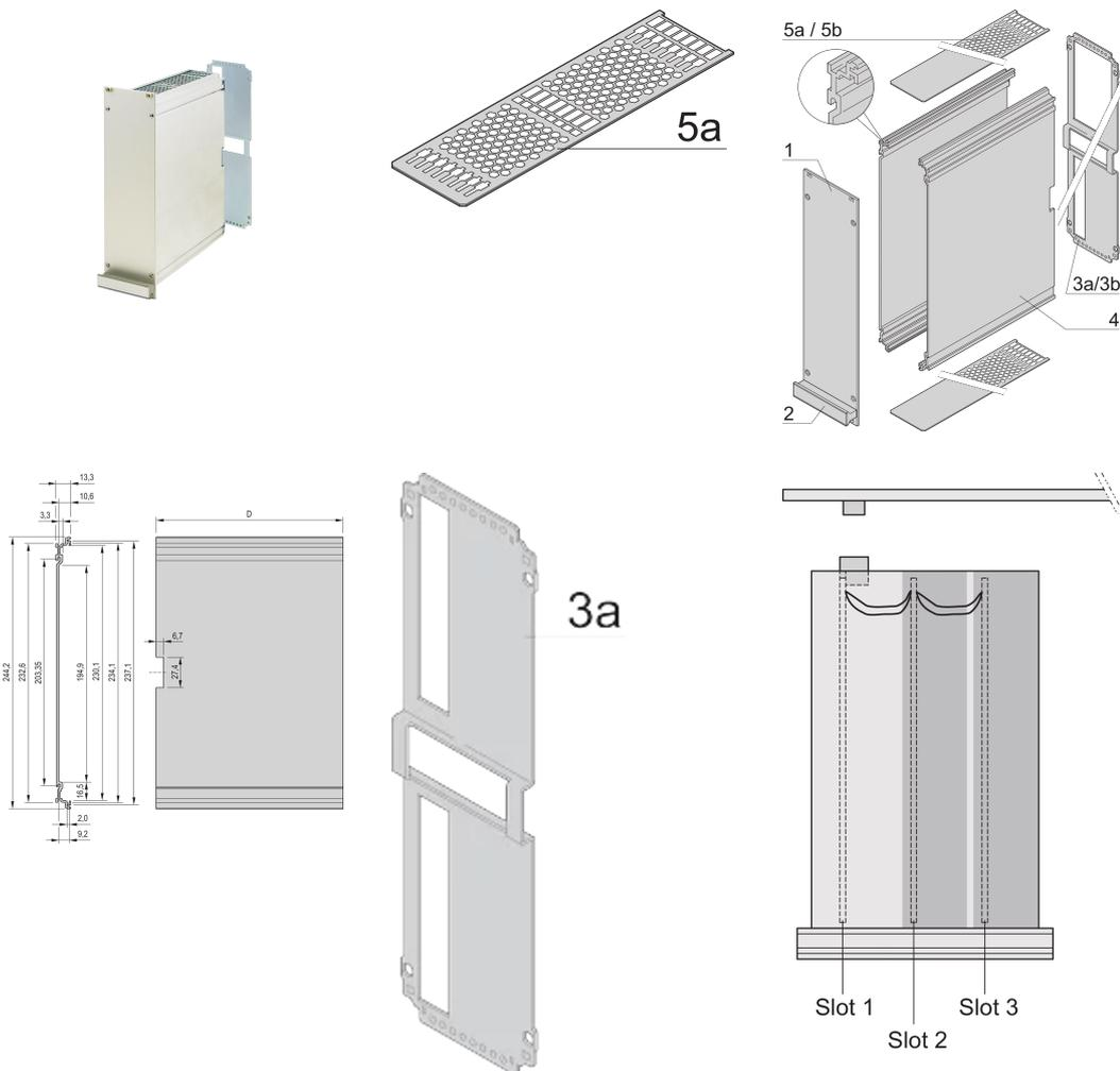
Frame type plug-in unit, non-shielded, perforated top / bottom cover, rear panel with cutout for one connector.
