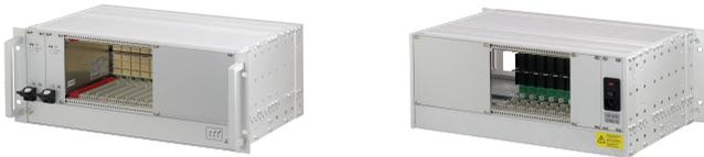
4 U CompactPCI Serial R3.0 System, with vertical Card Cage for nine 3 U Boards and one 3U Pluggable Power Supply.
